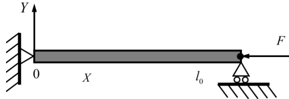
Figure 4.1 Model of a simply-supported inflating beam subjected to axial compression load.
